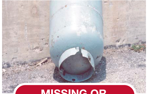
MISSING OR DAMAGED FOOT RINGS
