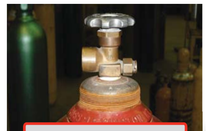
MISSING CYLINDER CAP
