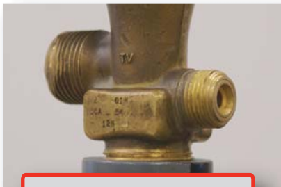
MISSING PRESSURE RELIEF DEVICE
